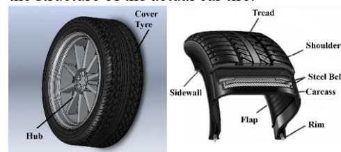
Figure 11 The structure of the car tire
